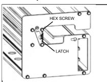
**1.** Loosen hex screw to allow Face Strip Retaining Latch to rotate out of the way. Insert Face Strip, reposition Latch and tighten screw.
