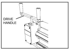
**6.** Using the handle, move the lacer head across the belt width at a smooth speed.
