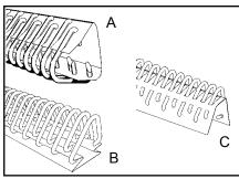
**4.** If using hooks as shown in A or B, remove carding paper at this time. If using hooks as shown in C, remove carding paper after installing hooks.
