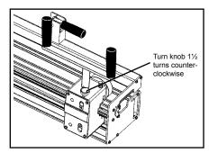
5. Return lacer head to end of lacer and turn adjusting knob  $1\frac{1}{2}$  additional turns counter-clockwise.
