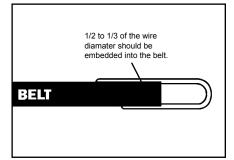
7. Turn adjusting knob counter-clockwise 1/2 turn and return head across the belt. Repeat until hooks are embedded 1/3 to 1/2 into the belt.
