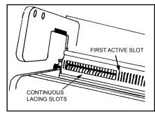
**3.** Insert hooks into the first active slot of the face strip. Secure with lacer pin.
