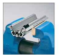
The Clipper® Vise Lacer is the ideal lacing tool for the user with only a few conveyor belts, while providing the reliability and performance of a machine splice. It is also easy to use and inexpensive.
